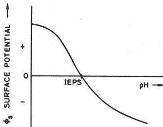
Figure 4. Schematic plot of surface electrical potential (zeta potential) as a function of fluid pH relative to the surface isoelectric point (IEPS).
